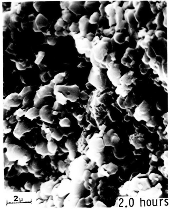
Figure 15. FRACTURE SURFACE SEM OF 30 m/o AlN, CARBON FURNACE, NITROGEN, 1605°C
