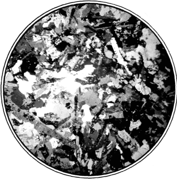
A. Andesite inclusion from the Flavrian mass in which the original trachytic texture and feldspar laths can still be seen, showing some replacement by quartz. x14
