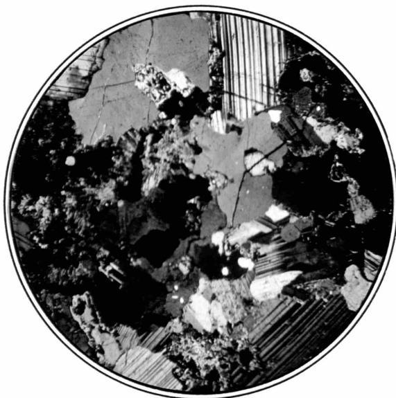
A. Quartz-gabbro, showing the fresh nature of hornblende and of plagioclase. x15
