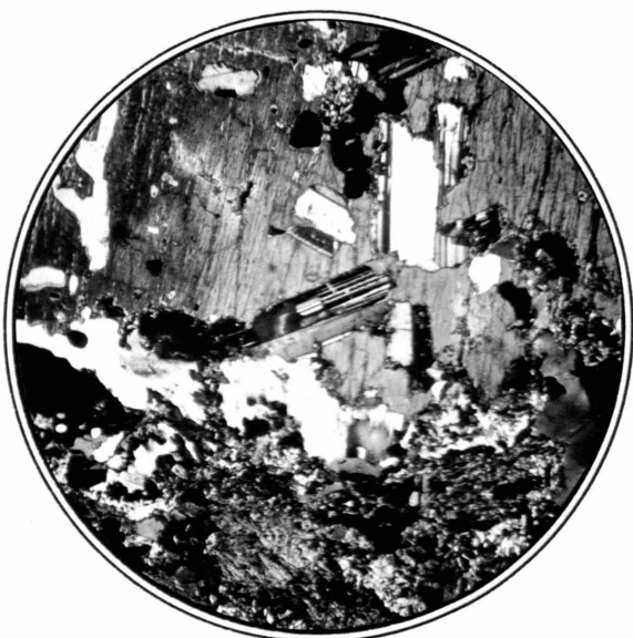
C. Quartz-gabbro, showing fresh hornblende with poikilitic inclusions of labradorite and slight embayment by primary quartz. The lower part of the field is unaltered pyroxene. x17
