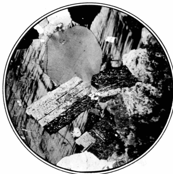
D. A section of the core phase from the Taschereau mass showing a large unit of microcline enclosing quartz and plagioclase. x20
