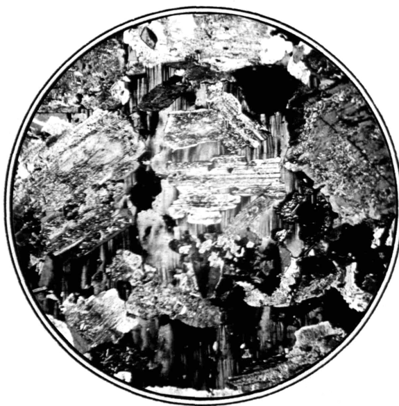
Plate XIV. Corroded and saussuritized plagioclase rimmed by clear albite and poikilitically enclosed in perthitic feldspar. xl4
