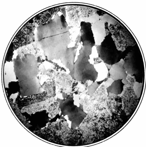
C. A section of the core phase showing the abundant nature of the quartz and four separate areas of microcline that extinguish together. x10
