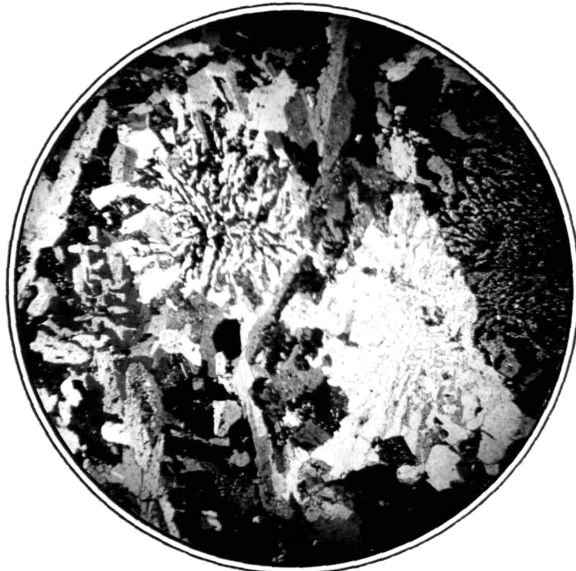
B. An inclusion still recognizable as andesite in which the quartz forms crude pseudographic replacement textures. x14
