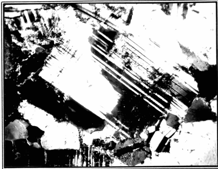
A. Fresh combination carlsbad-albite penetration twin of labradorite (Ab 47 An 53 ) in quartz-gabbro. x33
