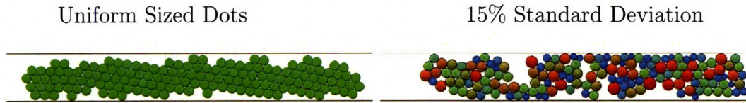
Figure 2-3: a) Shows the results of our simulation for 150 uniform sized quantum dots confined in a grating. The packing is hexagonally close-packed except for a few defects and grain boundaries. b) Shows the results of our simulation for 150 quantum dots whose diameters are determined by a Gaussian distribution with standard deviation equal to 15% of the mean radius confined in a grating. The dots are colored such that larger dots are more red, mean sized dots are green, and small dots are more blue. The dots are more cohesive because confining them increases the number of collisions and reduces the average kinetic energy.
