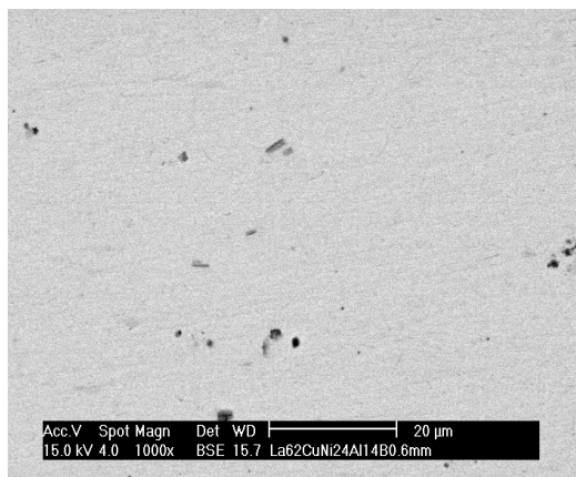
Fig. 9 (c). SEM Pictures of L62 alloys prepared by Bridgman solidification with growth rate of 0.6 mm/s.
