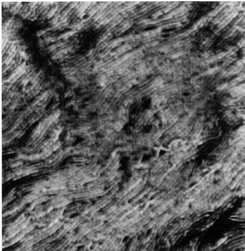
Figure 5.6. AFM phase image of crosslinked E30CL36 at 80% polymer concentration; image size is 1\mu\text{m} \times 1\mu\text{m} , and a domain size of the lamellae is 23nm (dry sample).
