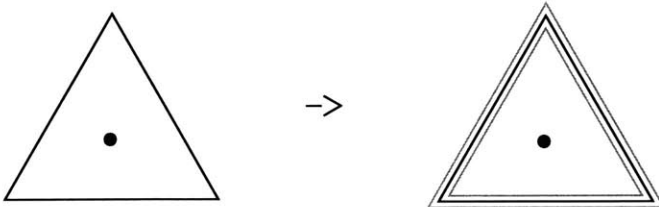
Figure 3-20. Rule 2b. Scale the implied shape up 110% and down 90% from the center to create the parameter space guide shapes for perturbing the implied shape. Here the guide shapes are in light grey.
