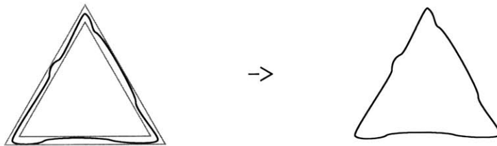
Figure 3-25. Rule 3d. Remove the guide shape to leave the final parameterized shape.
