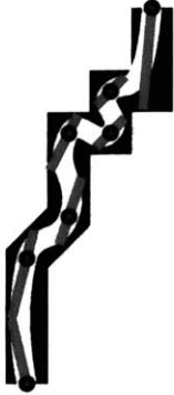
Figure 4–24. Raw hand–drawn stroke data and its conversion to a piecewise Bézier. The black polyline is the original data; the white piecewise Bézier is the curve representation before maximization. Tangents to the joints of the pieces are shown in grey and circles mark the joints themselves.
