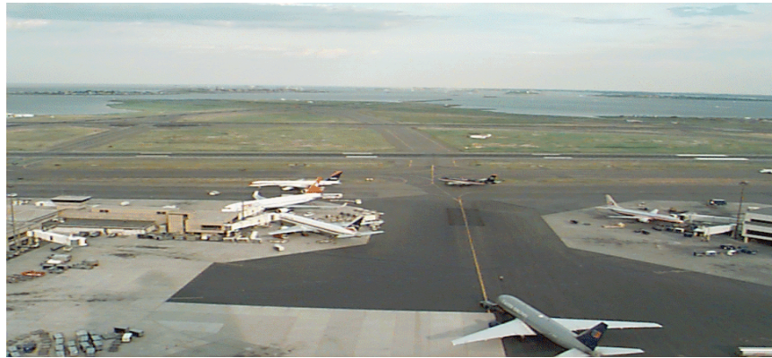
Figure 3.50: Taxiway blocking by pushback (A pushback on a taxiway blocks the taxiway while another taxiing aircraft is routed around it.)
