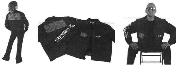
Figure 4-11: An embedded matrix of fabric-friendly LEDs enables the display of Nyx clothing.
