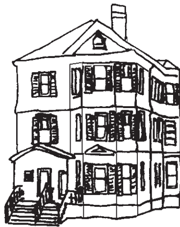
Figure 16. The more romantic, gable-roofed Roxbury tradition of three-decker house design identified by Krim. This is in contrast to the flat-roofed South Boston three-decker prototype (Chapter 1, Figure 2).
