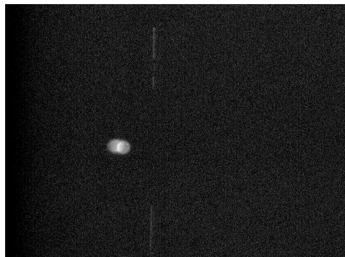
Fig.7 An infrared near-field pattern of an InGaAsN/GaAsN triple quantum well laser diode.
