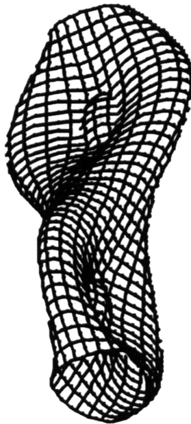
Figure B-1: Circular Cylindrical Shell in an ( n=2 , m=2 ) Buckled Configuration
