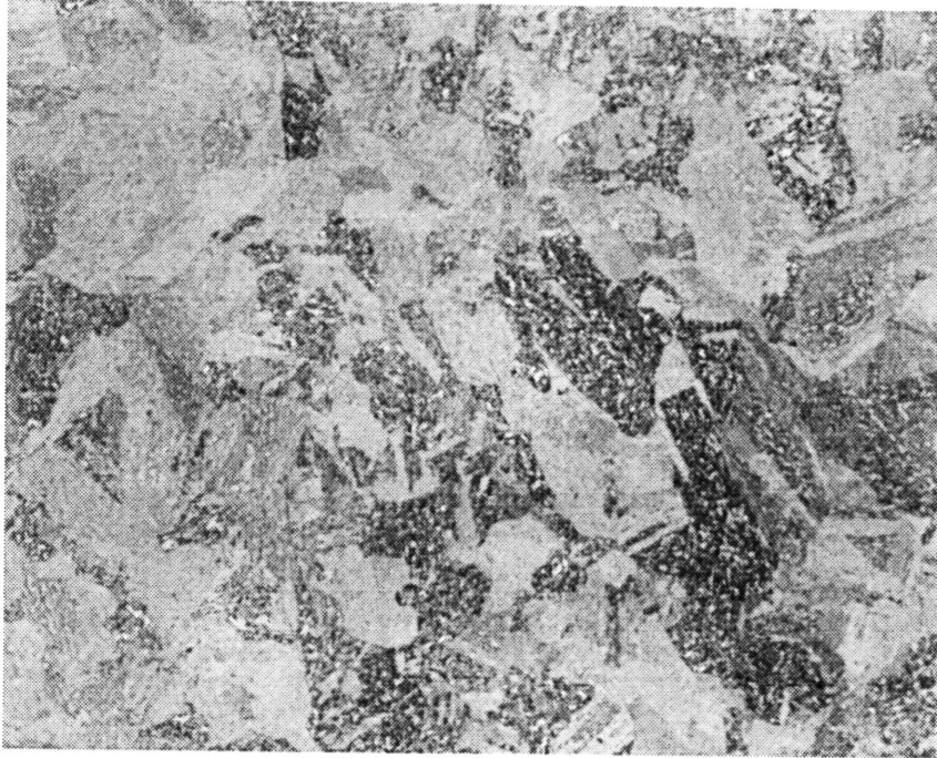
Figure 5.59 Microstructure of As-Received Material, Revealed by Etching with Nital Spec. 4-5-3, AR, Nital, Metallograph, 50X
