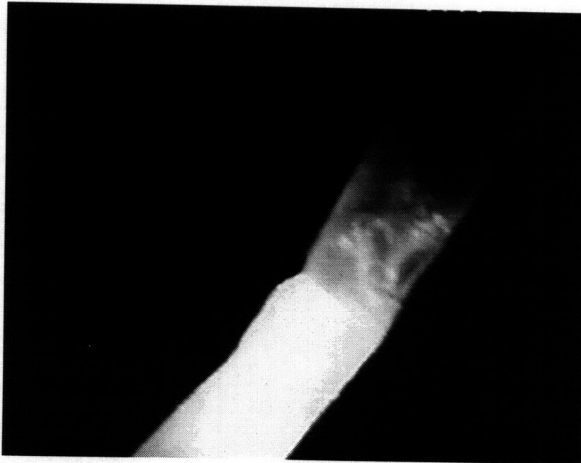
Figure 5.87 Dark-Field Image of Extracted Rod Exhibiting Contrast Boundary Possibly Due to Crystal Grain Boundary Spec. 4-2-1, 1250°C, 2°C/min, TEM
