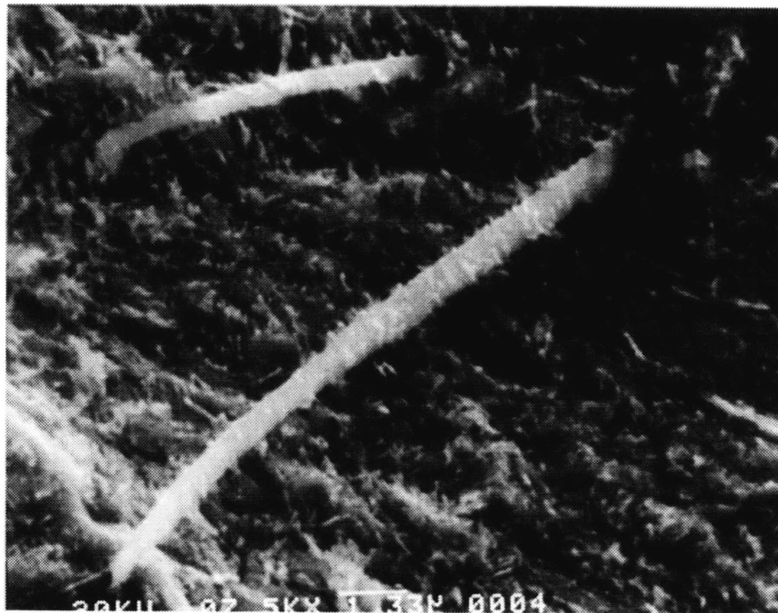
Figure 5.79 High-Magnification View of Rods As Revealed by Warm 50% Nitric Acid Deep Etch Spec. 4-2-2, 1250°C, 2°C/min, Warm Nitric, SEM
