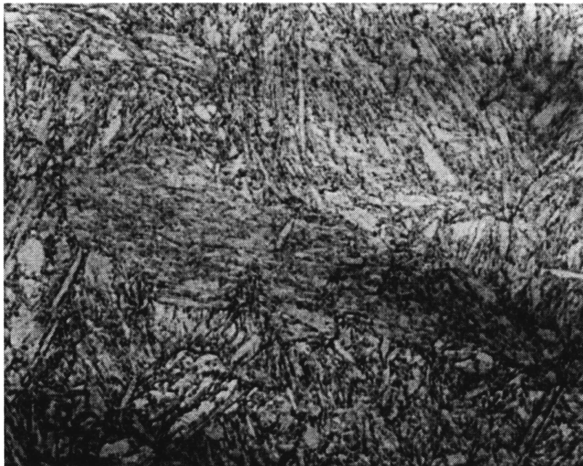
Figure 5.67 High-Magnification View of Structure of Air-Quenched Material, Revealed by Etching with Nital Spec. 4-2-3, 1250°C, AQ, Nital, Metallograph, 1000X
