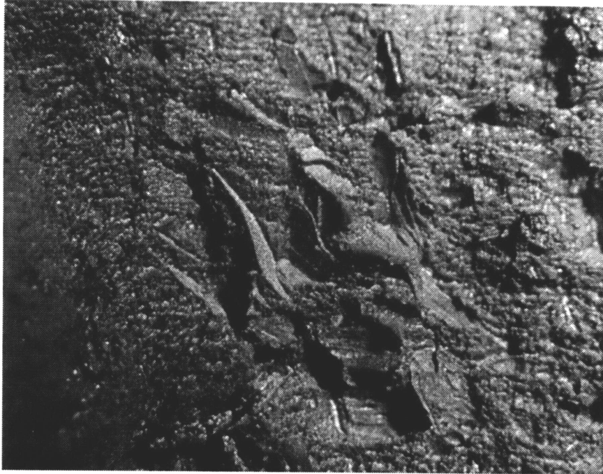
Figure 5.3 Optical Micrograph of Distorted Facets on As-Received Control Material Spec. 1-1-2, AR, Optical Fractograph, 20X
