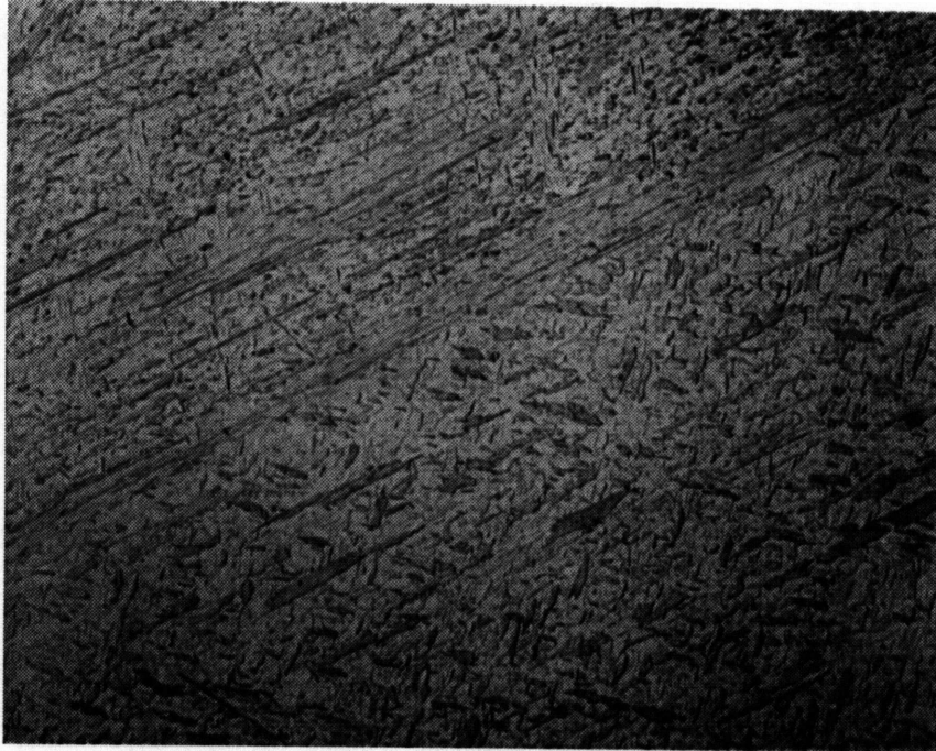
Figure 5.69 Lathe Martensite Morphology Revealed by Etching with Nital Spec. 5-1-1, 1300°C, 2°C/min, Nital, Metallograph, 200X
