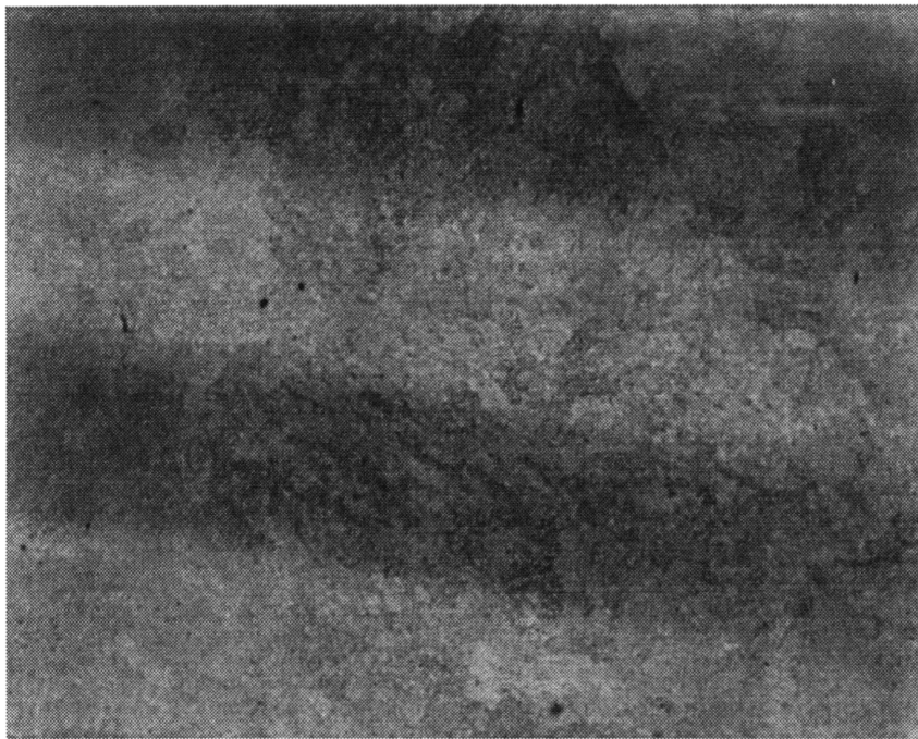
Figure 5.68 Low-Magnification View of 1200°C Control-Cooled Material With Small Prior Austenite Grains, Revealed by Etching with Nital Spec. 4-1-3, 1200°C, 2°C/min, Nital, Metallograph, 50X
