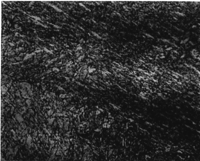
Figure 5.65 High-Magnification View of Structure of Control-Cooled Material, Revealed by Etching with Nital Spec. 4-2-2, 1250°C, 2°C/min, Nital, Metallograph, 1000X
