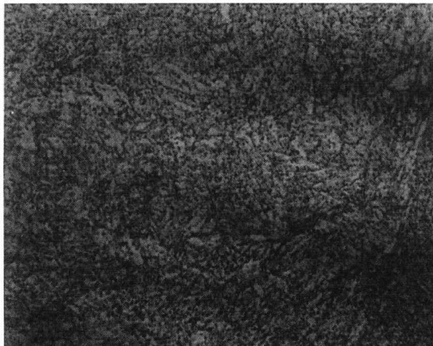
Figure 5.63 High-Magnification View of Microstructure of Quenched and Tempered Control Material Spec. 4-5-2, AR+QT, Nital, Metallograph, 500X
