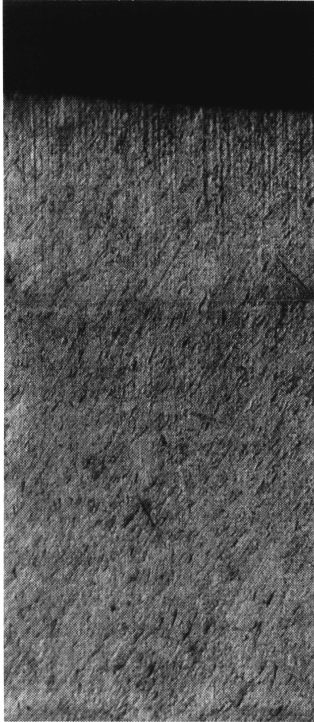
Figure 5.95 Composite Micrograph of Etched Surface of Figure 5.91 (Surface B), Etched With Vilella's Reagent, Showing Common Edge at Top and Rod Trace at Lower Center
