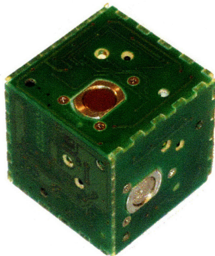
Figure 3-1: Each module in the system is a cube which measures 1.77 inches on each side and weighs 4.5oz. Each module is completely autonomous and can operate for several hours under its own power.
