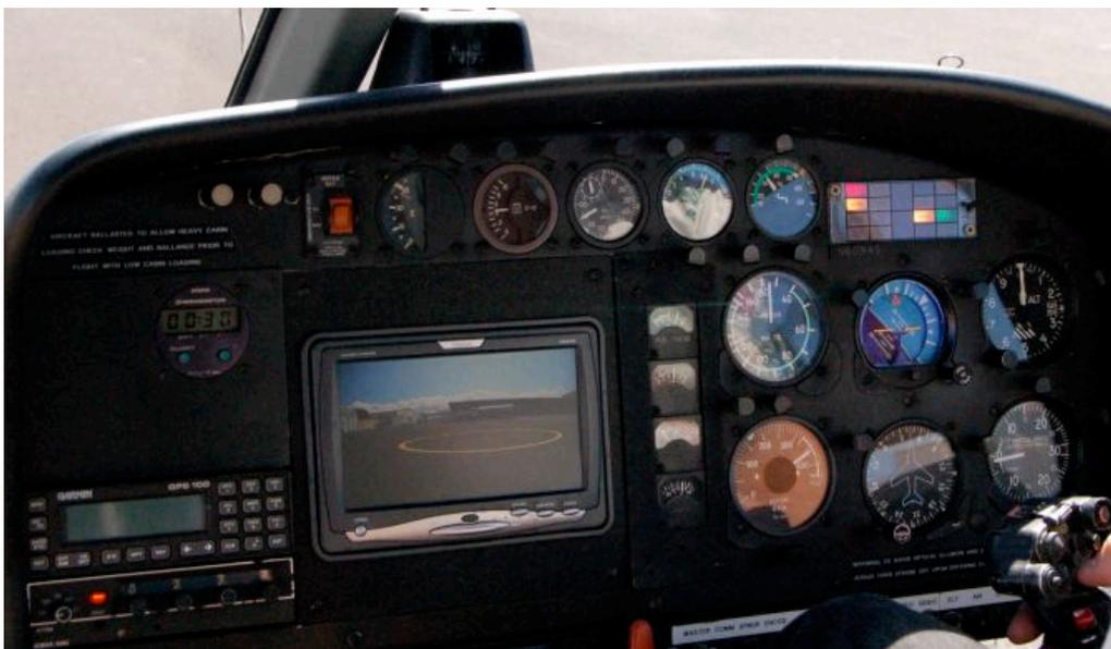
**Figure 7: Air tour helicopter panel with video monitor**
