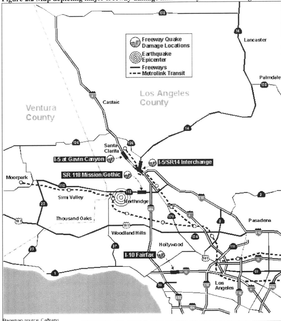
Figure 2.2 Map depicting major freeway damage immediately after Northridge.
