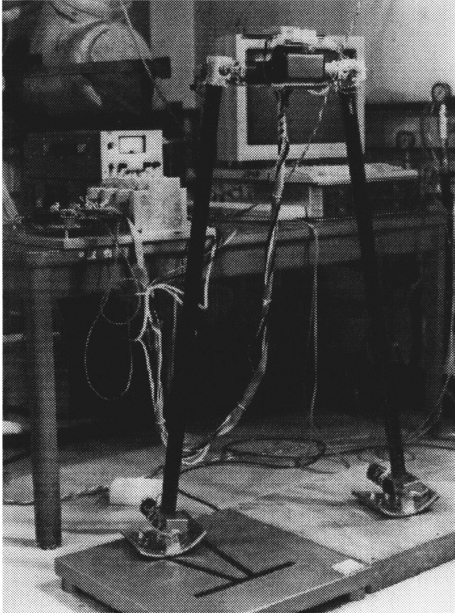
Figure 2-3: GeekBot test setup. The foot on the left is standing on the forceplate. Behind the robot is one of the transputer nodes, the Copley amplifiers, the electrical power supplies, and the Sun 3 workstation.
