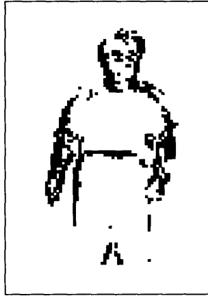
Figure 4-6: Due to the man's untextured clothing, motion is only detected around the outside of the man the takeh sequence and not in the interior. This closeup shows the motion pixels detected in image 27, run at half resolution. The motion pixels have fragmented and have been grouped into two connected regions.
