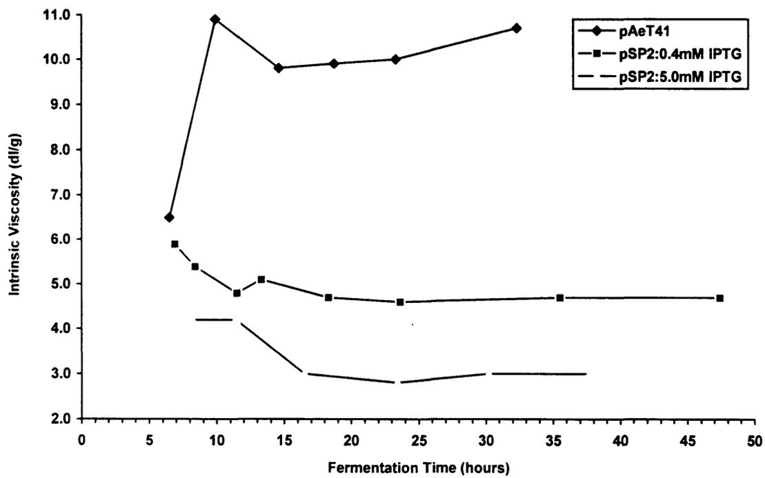
**Figure 6.** Intrinsic Viscosity in Chloroform (30°C) of PHB Produced by Recombinant *E. coli* (10 Liter Fermentations)
