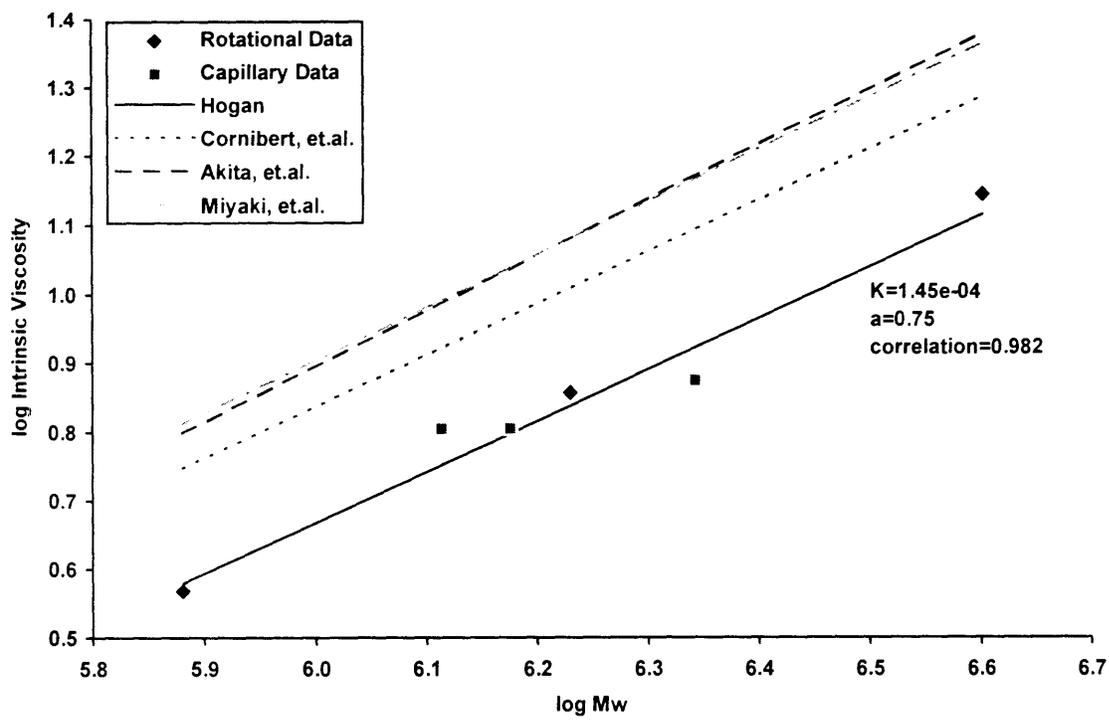
Figure 19. Intrinsic Viscosity-Molecular Weight Relationship for PHB in Trifluoroethanol at 25°C
