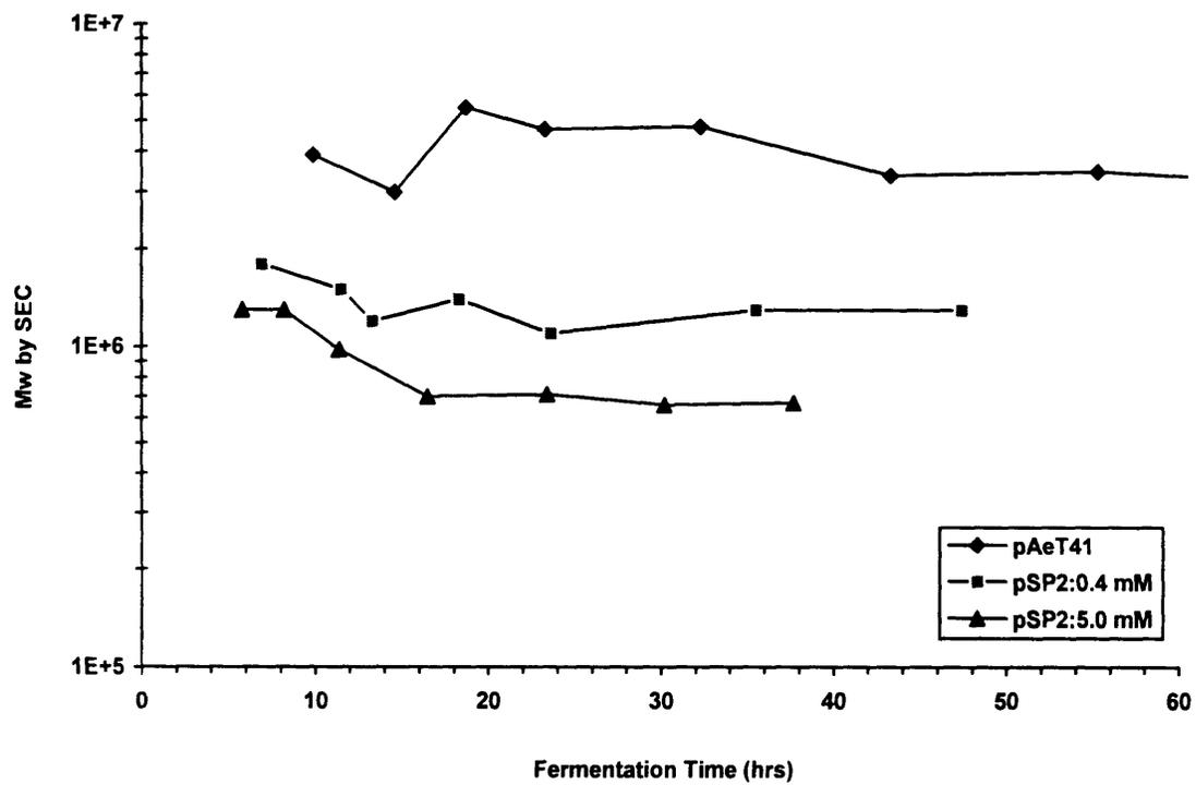
**Figure 9.** Weight-Average Molecular Weight of PHB Produced by Recombinant *E. coli* Determined by SEC (10 Liter Fermentations)
