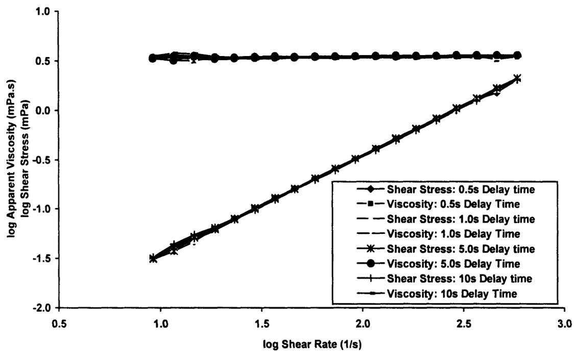
**Figure 20.** Time Dependency of Viscosity of PHB in TFE at 25°C
