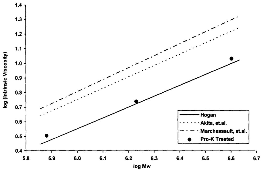
**Figure 21.** Intrinsic Viscosity-Molecular Weight Relationship for PHB in Chloroform at 30°C, Including Proteinase-K Treatment
