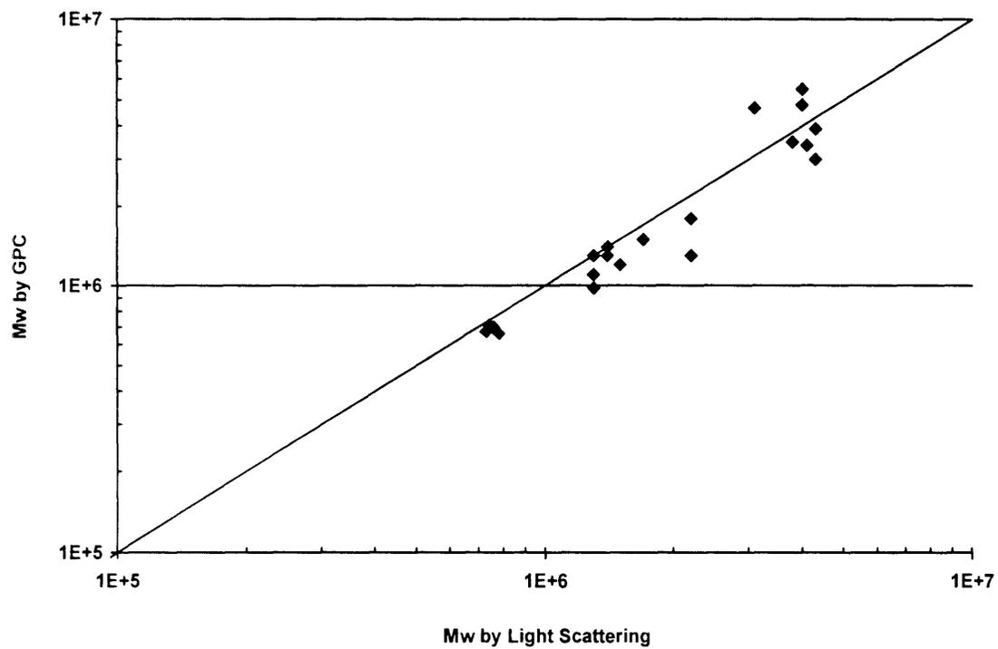
**Figure 17.** Comparison of Light Scattering and SEC Data
