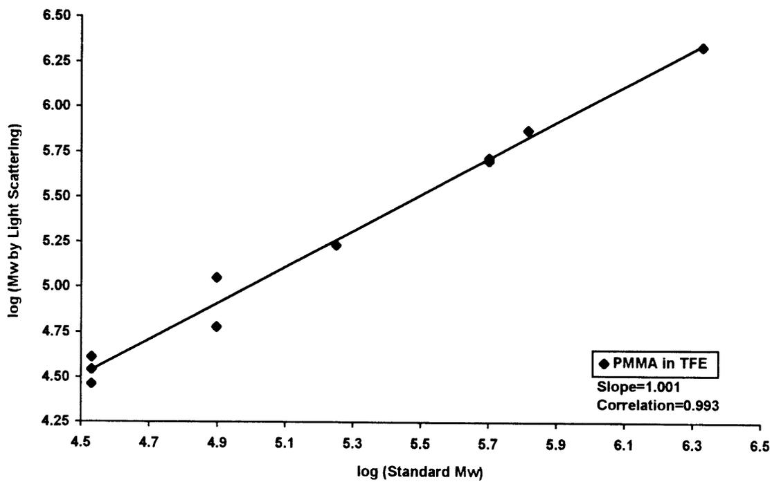
Figure 4. PMMA standards.  $dn/dc=0.198$
