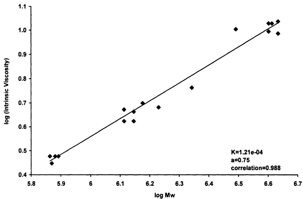
**Figure 15.** Intrinsic Viscosity-Molecular Weight Relationship for PHB in Chloroform at 30°C
