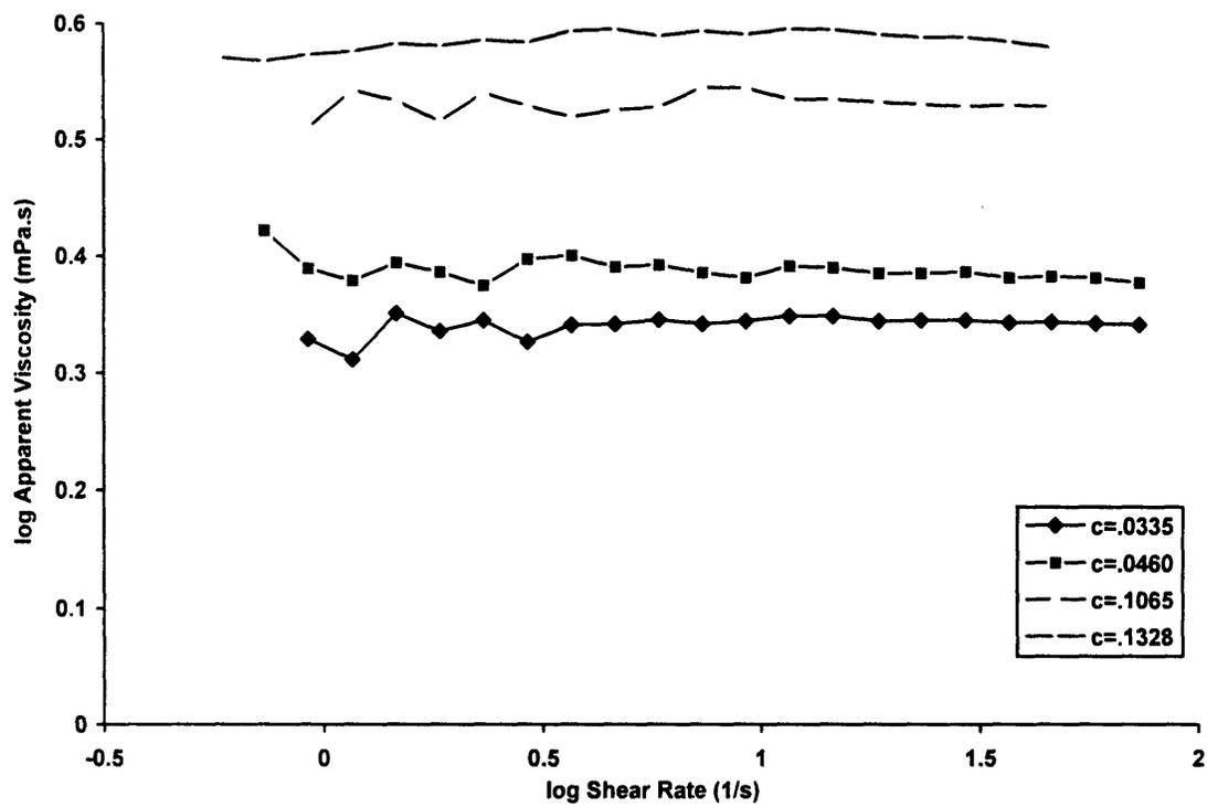
Figure 18. Viscosity as a function of Shear Rate for  $M_w=1.7 \times 10^6$  PHB. Concentrations from 0.0335 to 0.1328 g/dl
