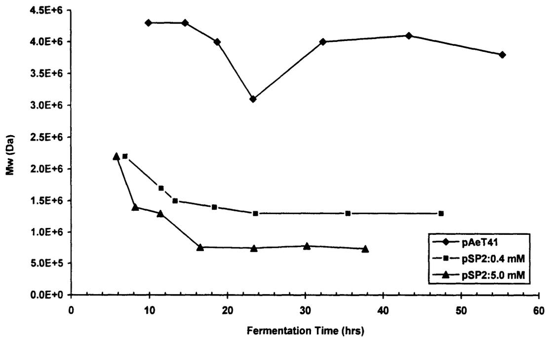
**Figure 12.** Weight-Average Molecular Weight of PHB Produced by Recombinant *E. coli* Determined by Light Scattering (10 Liter Fermentations)
