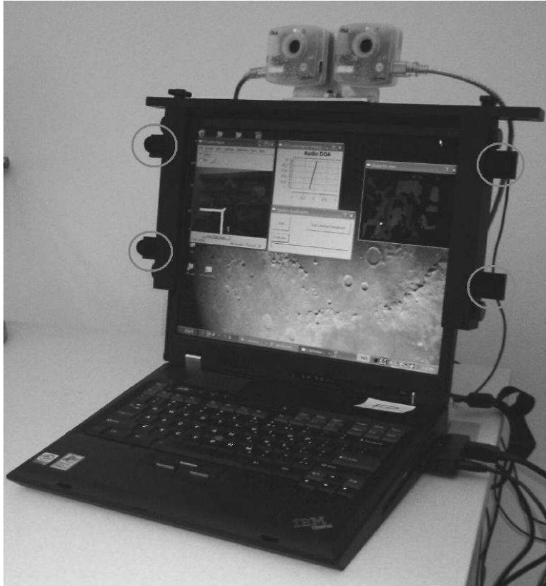
Figure 4-1: The microphone array setup used for all experiments on real data. Microphones (highlighted by grey circles) are held in a plastic frame surrounding the laptop screen. The top two microphones were used in all experiments.
