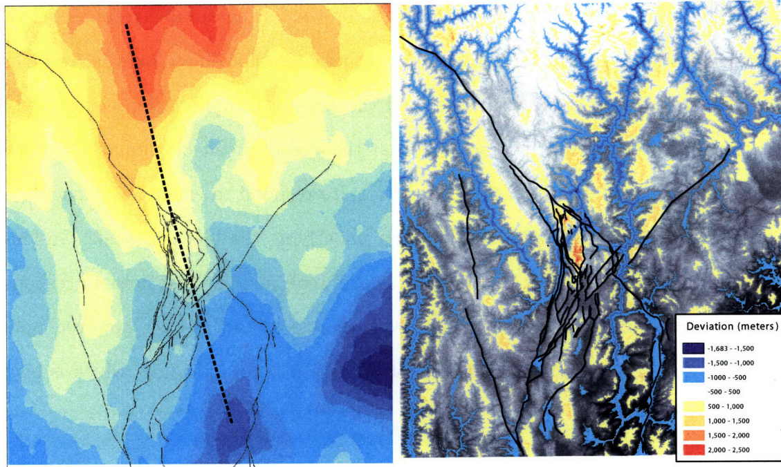
Figure 5-14: Left: Elevations smoothed by averaging over a 20km radius moving window. Right: Deviation of elevations from smoothed and averaged elevations superimposed over a grayscale image of the DEM. Areas in grayscale are within 500m of the smoothed and averaged elevations.
