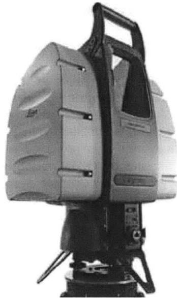
Figure 1.3. Leica model HDS3000 time of flight range scanner. Mounted on a tripod at a worksite, this range scanner pulses a laser beam and measures the time taken by the beam to bounce off the target and return to its source. Typical accuracies are on the order of 6mm over target distances of 50 m.
