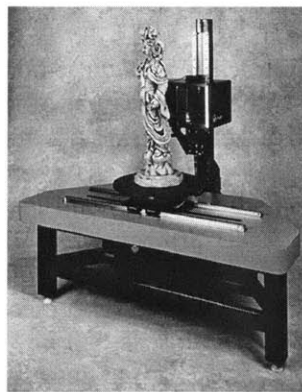
Figure 1.2. A typical laser scanner system, this Cyberware Model 3030 RGB/MS uses two linear and one rotational stages to capture full view 3D data from a target. Sampling pitch is 0.25-1.0mm in X and Y directions, and 50-200 microns in the Z direction. The translation table is approximately waist high.
