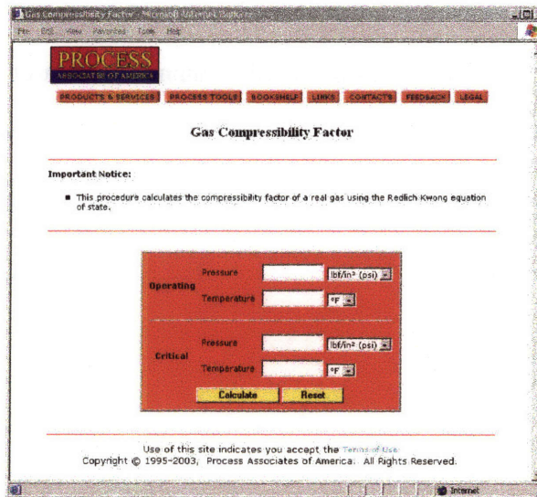
Figure 3-6 A web page that contains an executable interface of process tools
