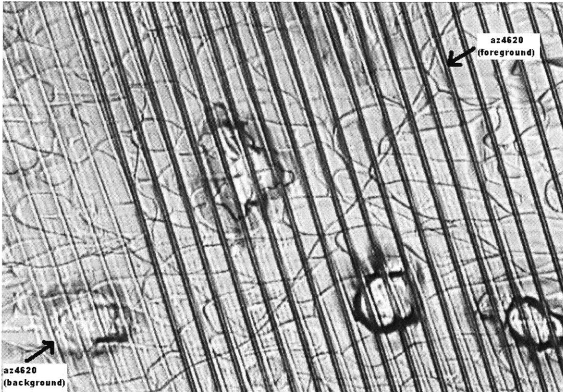
Figure 4.3: A top down view of the completed AZ4620 sensor showing the top and bottom features. Due to a misalignment error the features are not aligned properly (the separation of the features (parallel bars) is 100 microns). Note: the entire sensor has a reddish tinge (with cracks) to it due to a very thin layer of AZ4620 deposited over the entire 1 st and 3 rd layer of PDMS.
