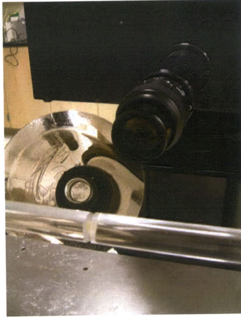
Figure 3-2: A Cordin 550 high speed digital camera is used to record the compression of the SHPB samples.
