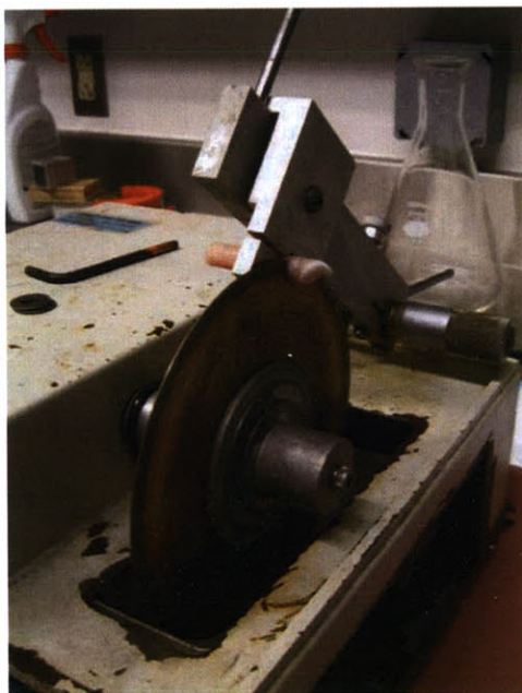
Figure 3-7: An irrigated diamond encrusted wafering saw is used to section the cores into orthogonal right cylinders.
