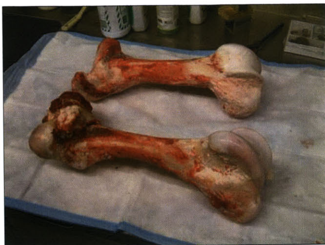
Figure 3-3: Intact bovine femurs are transported to the Orthopedic Biomechanics Laboratory at Beth Israel Deaconess Medical Center for machining.
