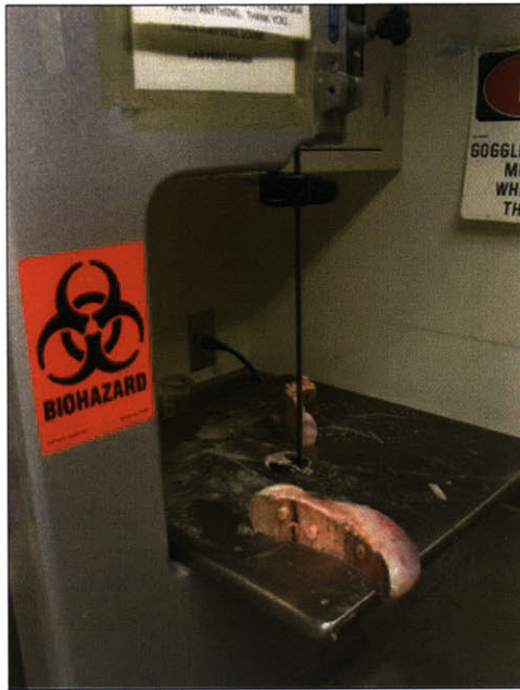
Figure 3-5: A cut is made perpendicular to the knee to release the trabecular cores.
