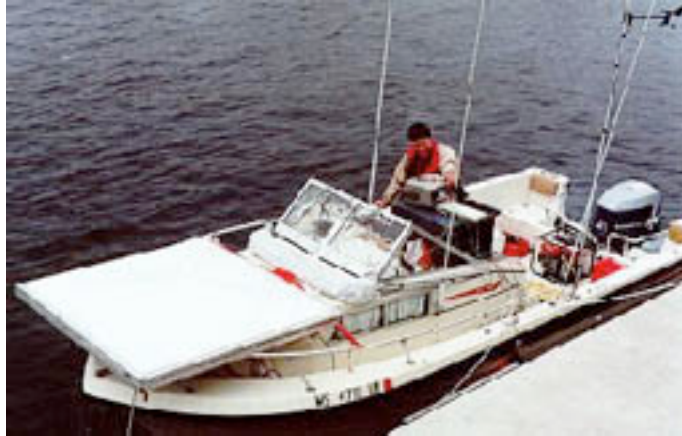
Figure 1.3 ProSensing's MBL-profiler rigged aboard a small boat
