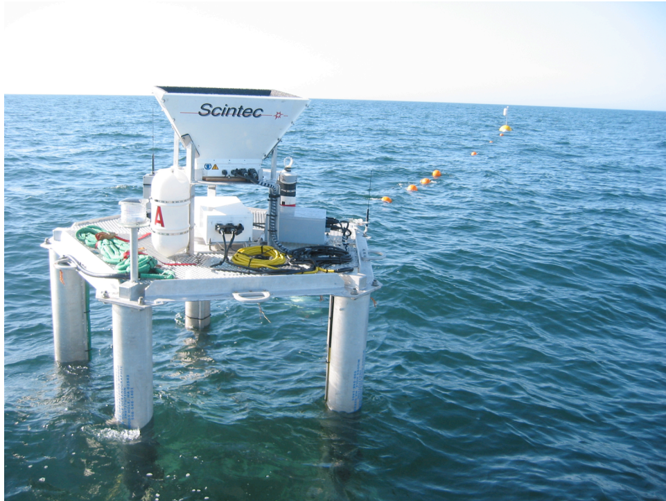
Figure B.5 A fully instrumented ASIS tethered to its surface mooring.
