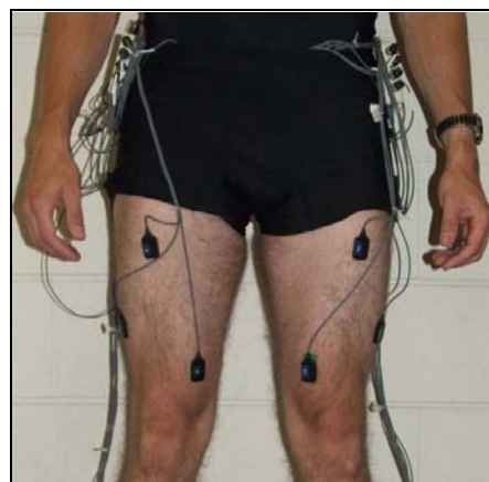
Figure 31. Electrode placement on the vastus lateralis, vastus medialis, and rectus femoris of the left and right leg. The EMG junction boxes are shown on the subjects left and right hip.
