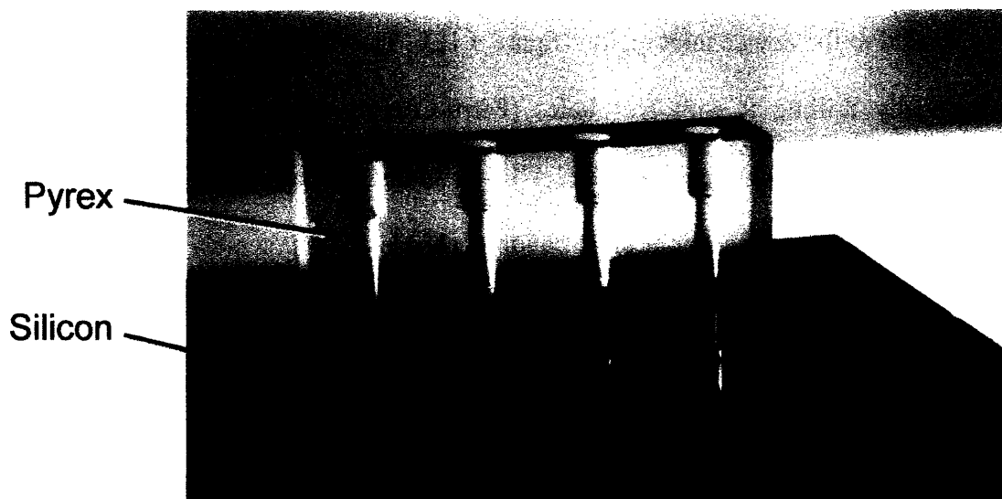
Figure 4.13: A drilled Pyrex piece (1 cm thick) anodically bonded to a silicon microreactor.
