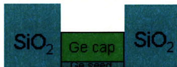
Figure 3.17 Schematic of the structure of SEG wafers. SiO 2 sidewalls were ~1μm deep. 99% of the wafer surface was covered by SiO 2 .
