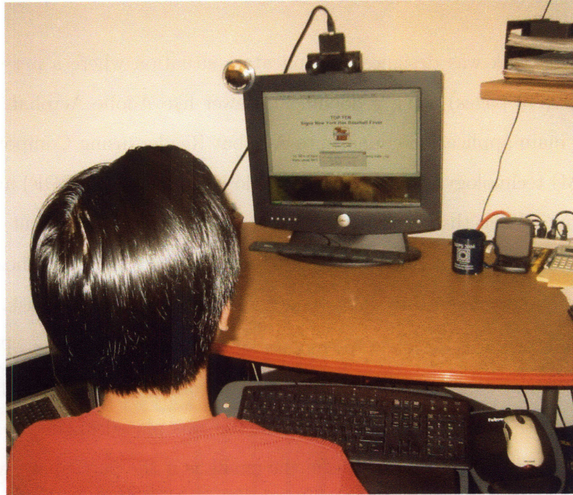
Figure 2-10: Experimental setup. A stereo camera is placed on top of the screen to track the head position and orientation.
