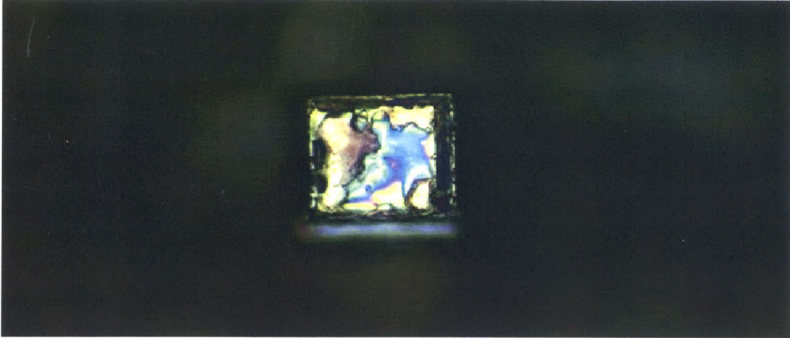
Figure 3-15: Micrograph showing the poor condition of the AuSn alloy on the top surface of an InP pillar after an unsuccessful bonding attempt.
