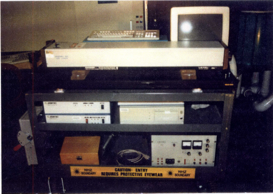
Figure 3.23: The laser Doppler velocimetry system. The emitter and sensor are connected to the laser via fiber optics.
