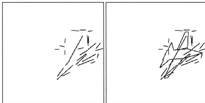
Figure 6-18: a) Selected segments b) Selected data aligned with model. As we can see, the alignment is not good enough and the object is NOT FOUND in the given scene. Alignment - score < 0.75.
