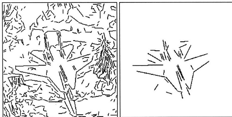
Figure 6-41: a) The segments in the image. b) The selected segments.
