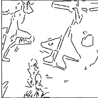
Figure 1-6: Foveated region after the stereo algorithm is run to determine where to fixate the eyes. Number of features = 300. Number of alignments = 300^3 * 20^3 = 10^{11} . Note that we are looking at a region of interest (region that could contain the model object) from the initial scene in greater detail.
