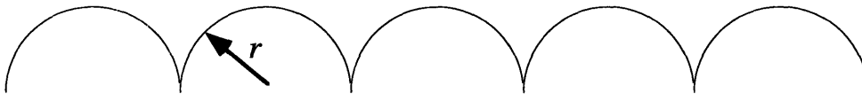
Figure B.1: Cross-section of the geometry assumed for a rough interface. The radius of the hemispherical caps that are used to model the rough interface is denoted r .
