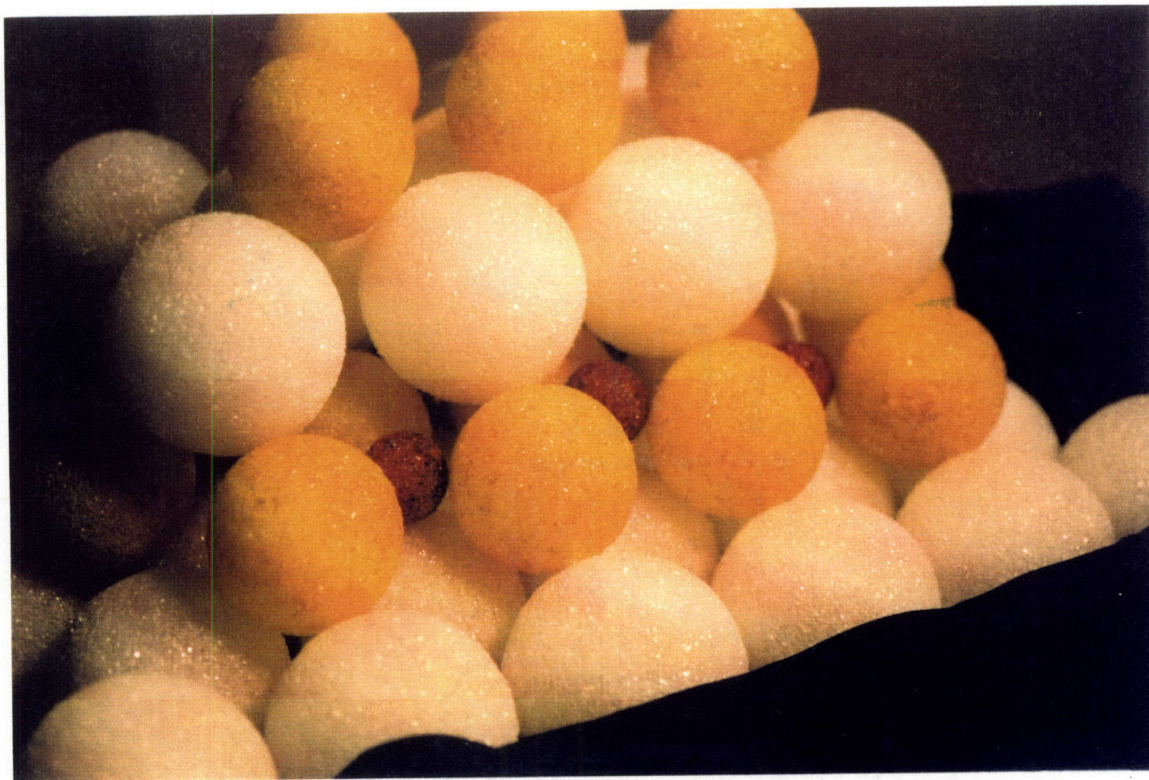
Figure 3.15: Structure of the \eta phase copper-tin intermetallic, \text{Cu}_6\text{Sn}_5 . The copper (yellow) and the tin (white) atoms are shown in the NiAs structure. The excess copper atoms would be located on one tenth of the tetrahedral interstitial sites indicated with the small red balls. The proper size ratio for copper to tin is used. Both \text{Ni}_3\text{Sn}_2 and \text{FeSn} also have structures based on NiAs.
