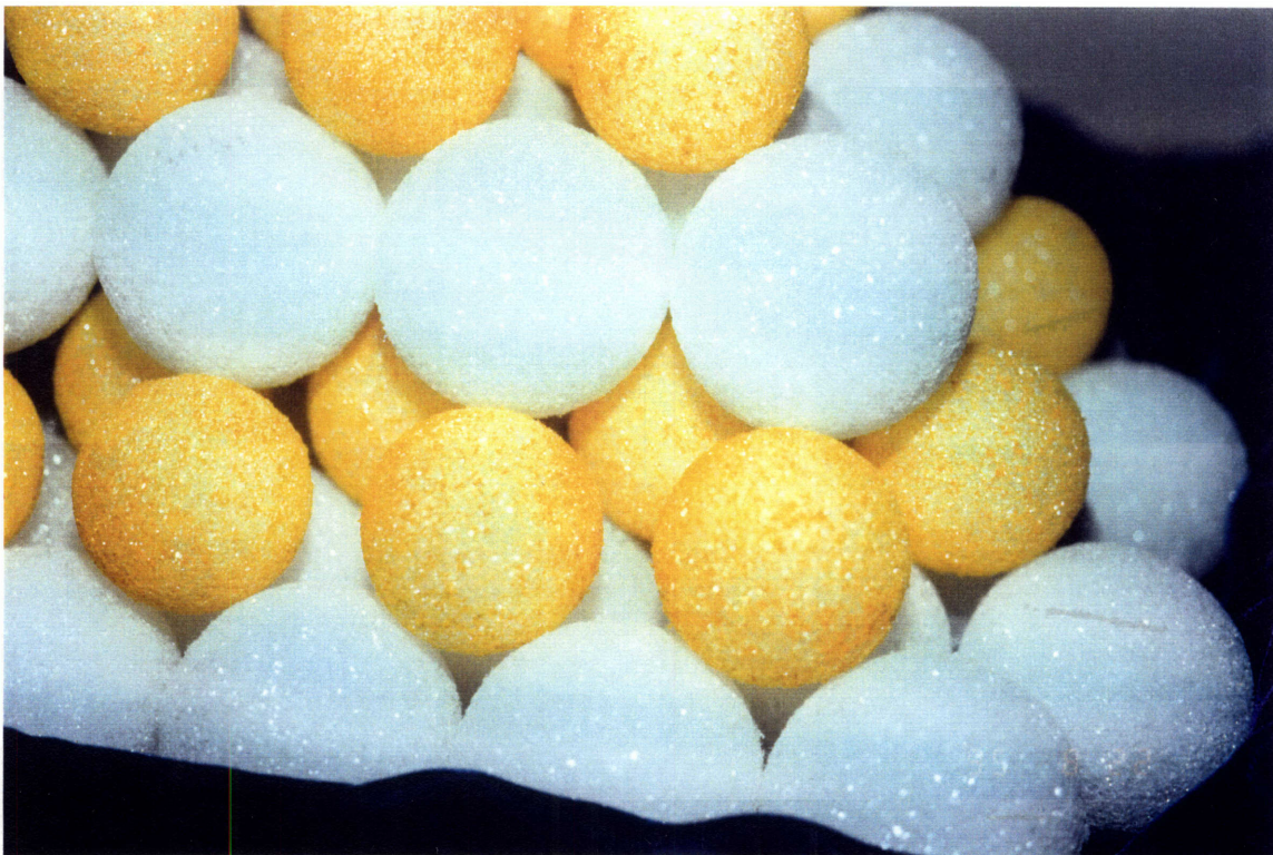
Figure 3.14: Structure of the \epsilon phase copper-tin intermetallic, \text{Cu}_3\text{Sn} . The lattice type is \text{Cu}_3\text{Ti} which has AB,A... hexagonal close packing. The yellow balls represent copper atoms, and the white ball are the tin atoms. The proper size ratio of copper to tin is maintained. Notice the space in the copper layer. \text{Ni}_3\text{Sn} also has this basic structure.
