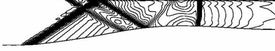
Fig. 1. Mach contours for steady flow through supersonic diffuser. Steady-state inflow Mach number is 2.2.
