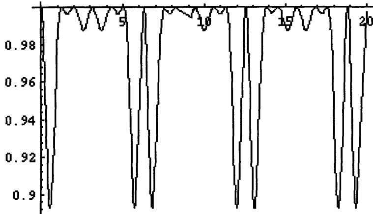
Figure 6.19 Initial magnetization was along Y. After spatial square wave modulated 90y pulse, the magnetization was spin locked along Y.
