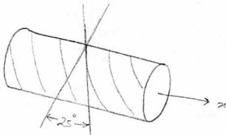
$$\begin{aligned}\sigma_{xx}' &= \frac{P \cdot \frac{\pi}{4} D^2}{\pi D t} \\ &= \frac{PD}{4t} = \frac{1 \times 750}{4 \times 10} \\ &= 18.75 \text{ MPa}.\end{aligned}$$
