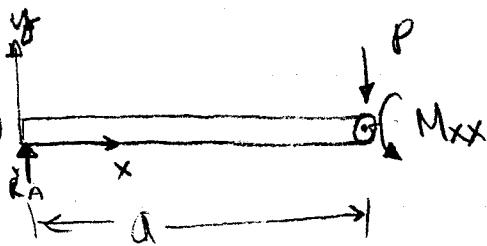
$$\begin{aligned} \sum F_y &= 0 & R_y^A &= P \\ \sum M &= 0 & M^A &= Pa \end{aligned} \quad ] \text{Reactions}$$
