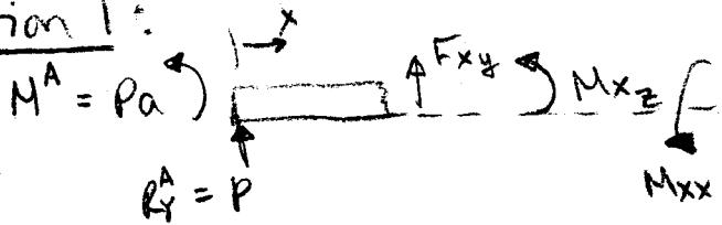
$$\begin{aligned} F_{xy} &= -P : \sum F_y \\ M_{xz} + F_{xy} \cdot x + Pa &= 0 \\ M_{xz} &= -Pa + Px \\ &= P(x-a) \\ x \approx 0 &\rightarrow = -Pa \end{aligned}$$
