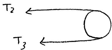
$$\begin{aligned} T_2 &= T_3 e^{\mu_1 \pi} \\ \Rightarrow T_3 &= T_2 e^{-\mu_1 \pi} \end{aligned}$$
