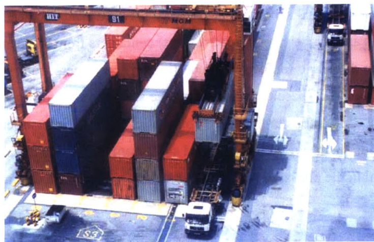
Figure 1-2. A RTG yard crane placing a container on a truck for transport to the quayside
