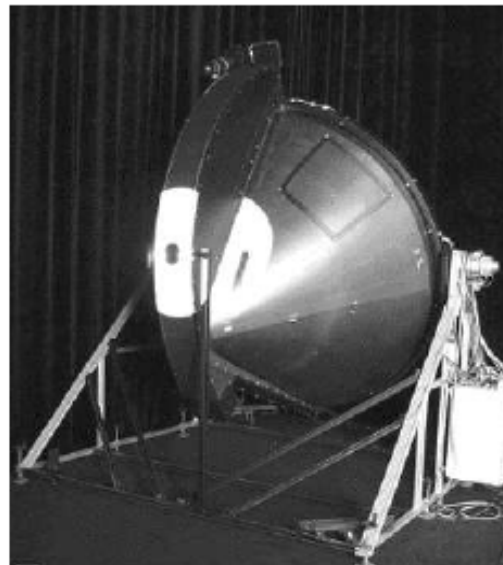
Figure 2.6 EPFL video-projection goniophotometer (Andersen et al. 2005a)
