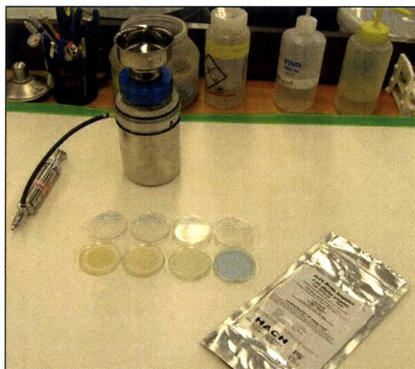
Figure 5.2 – Membrane Filtration apparatus (Mattelet 2006)
