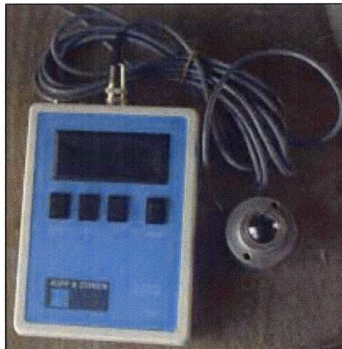
Figure 5.7 - Solar radiation measurement apparatus (Oates 2001)
