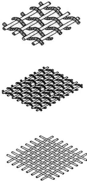
Figure 11: The loose plain weave, tight plain weave and laid weave of membrane yarns (Shaeffer, 1996)
