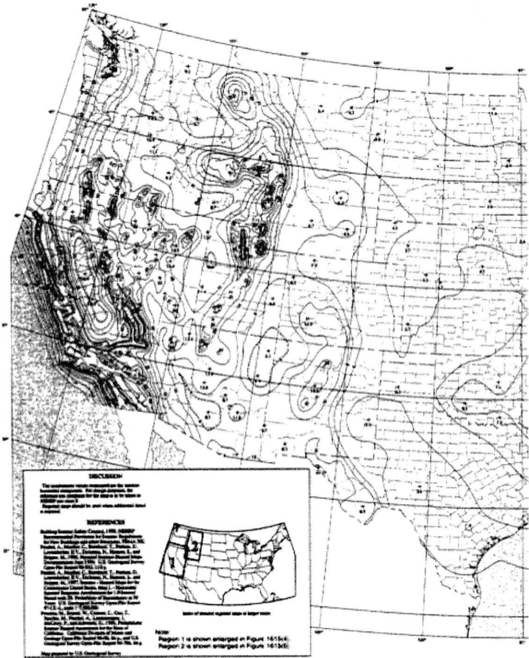
Figure 4-5: Maximum Considered Earthquake Ground Motion for 1.0 Second Spectral Response Acceleration, 5% Damping (Figure 1615(2) in 2003 IBC)
