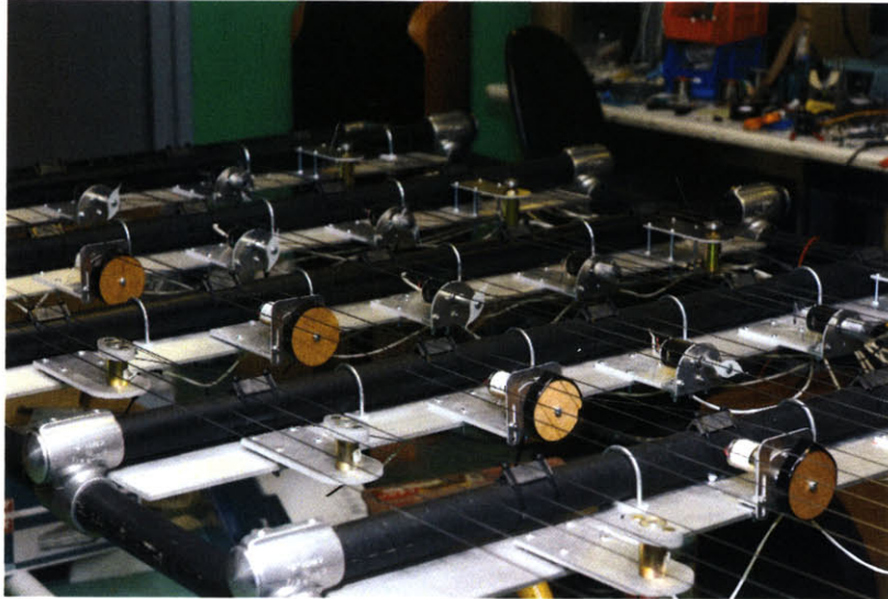
Fig. 4.19: The individual bridge assemblies are visible just next to each actuator.
