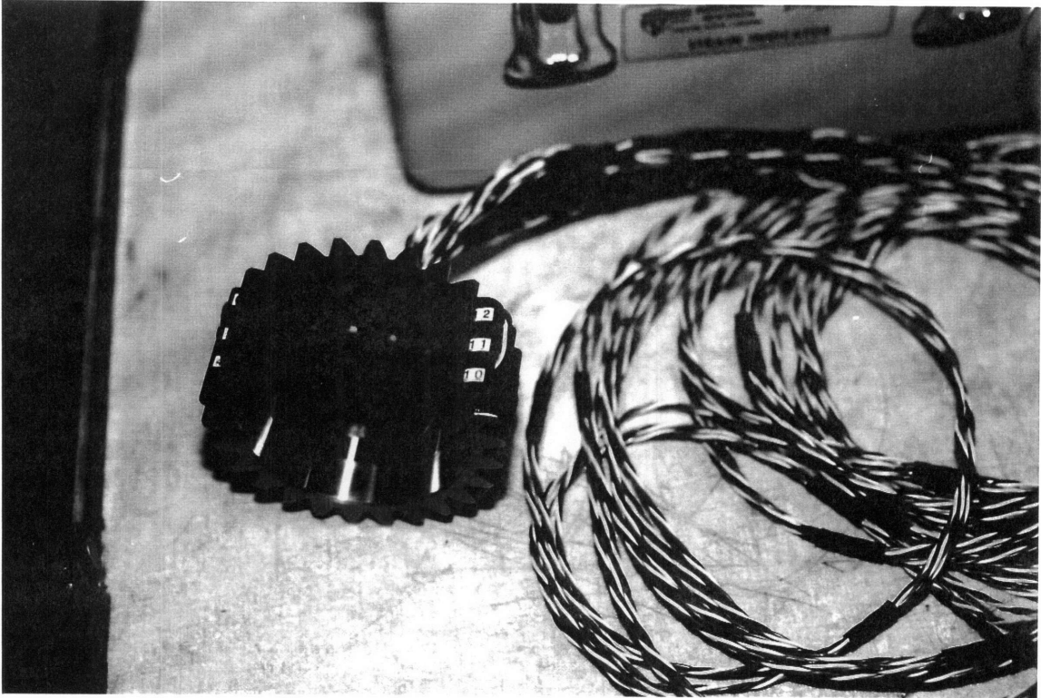
Figure 5.17: Illustration of the strain gauged gear with strain gauges 10 through 12 visible.
