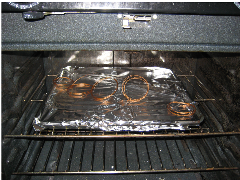
Figure D-2: A photograph of the quartz tube and thermocouples in the oven during a curing session.
