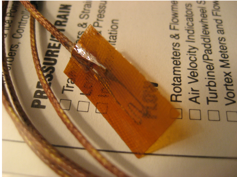
Figure 5-2: A photograph of one of the C01-K surface thermocouples showing details of the junction.
