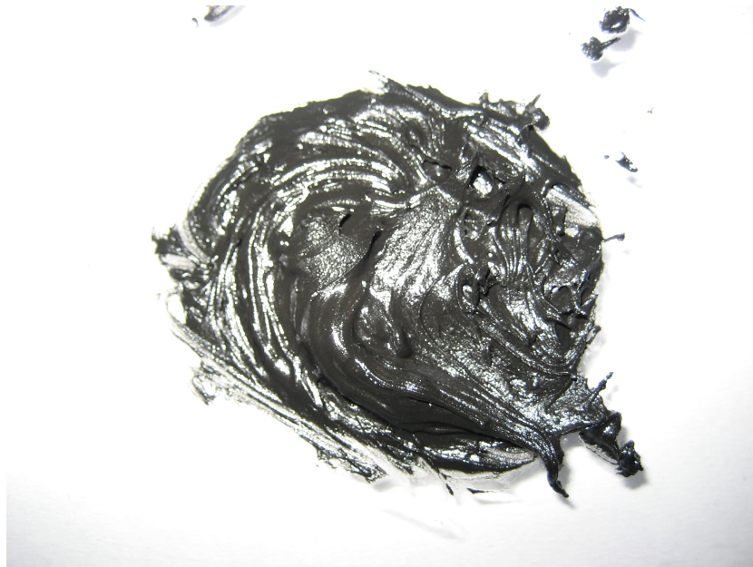
Figure D-1: A photograph of a properly mixed batch of OB-200 epoxy adhesive.
