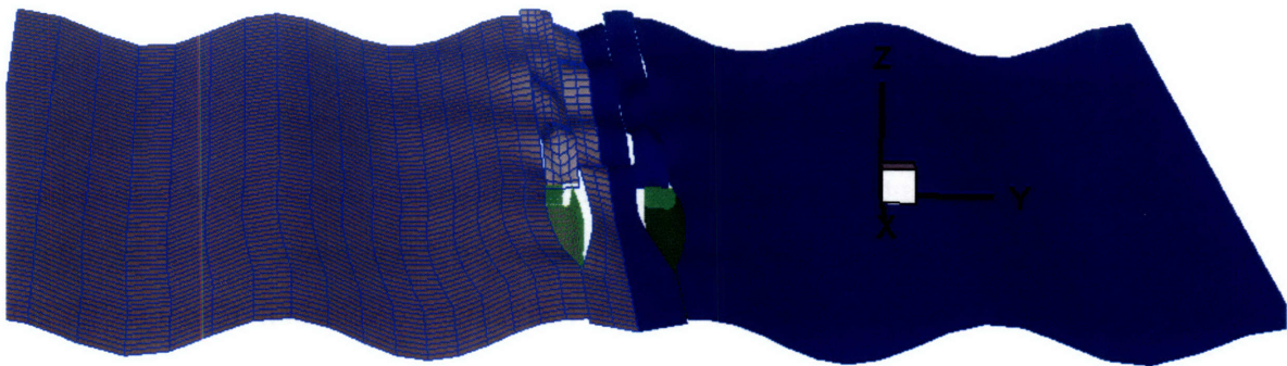
Figure 25 Semi-SWATH seakeeping simulation in beam seas at 18 knots
