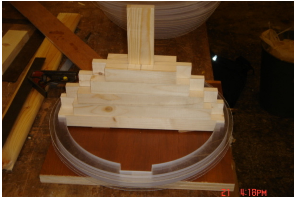
Figure C-3: The fixture that was made and used for alignment of the discs and flanges.
