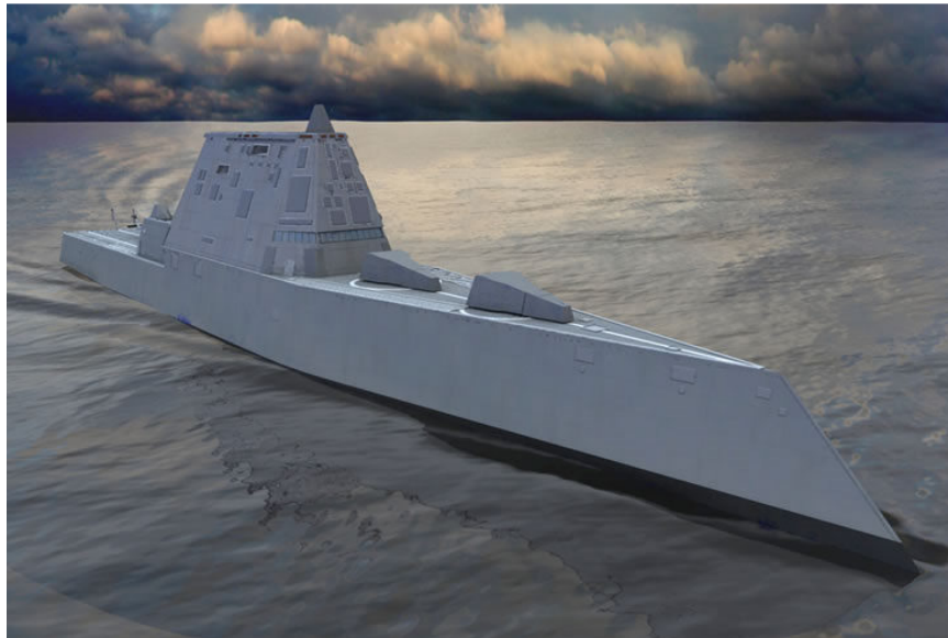
Figure 7-3: An artist's rendering of the next generation destroyer. This ship will have two 34.6 MW electric motors [45].
