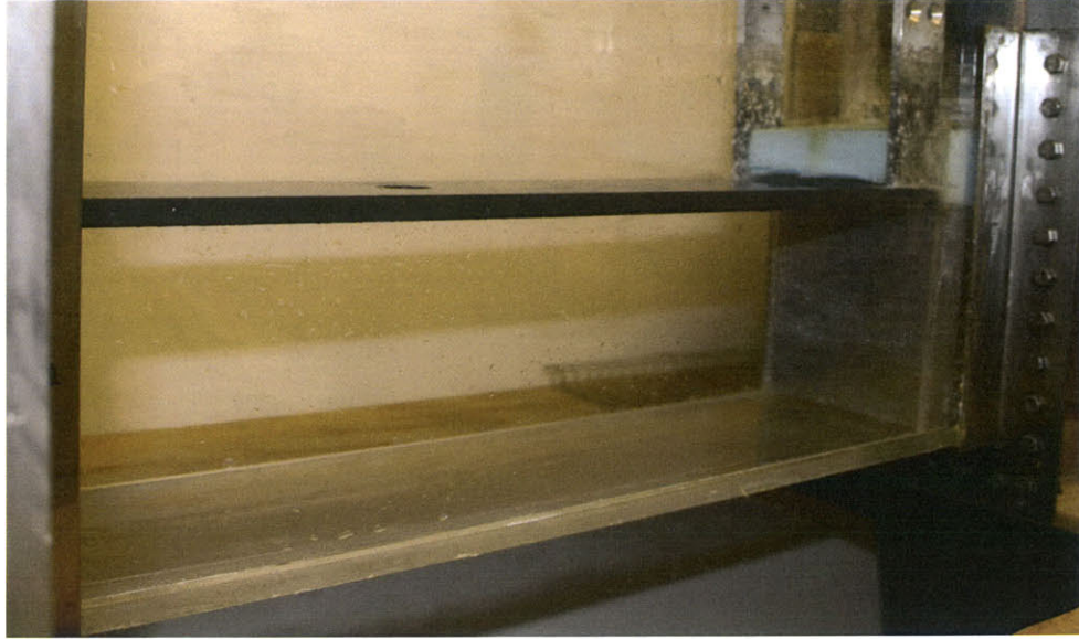
Figure 3-3: Flat plate model installed in water channel test section
