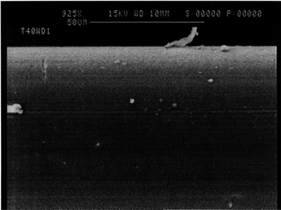
Figure 6-102: The Teftzel-Silicone-coated optical-fiber under 40 wet-dry cycles (925 X).
