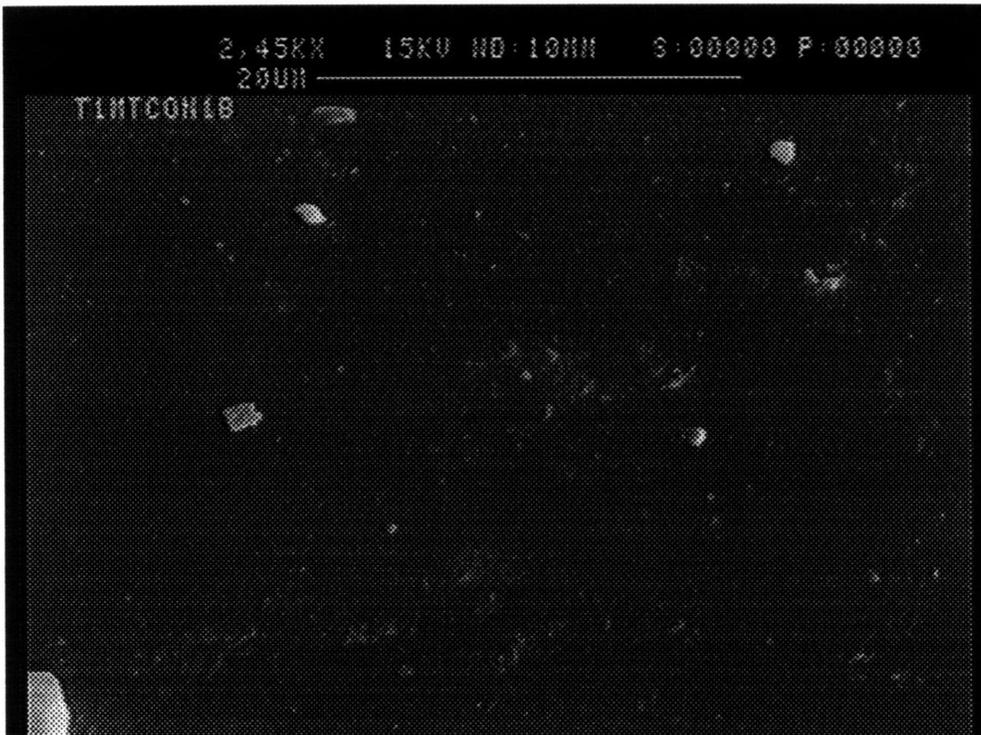
Figure 6-88: The Teftzel-Silicone-coated optical-fiber inside the cement paste for 1 month (2450 X).
