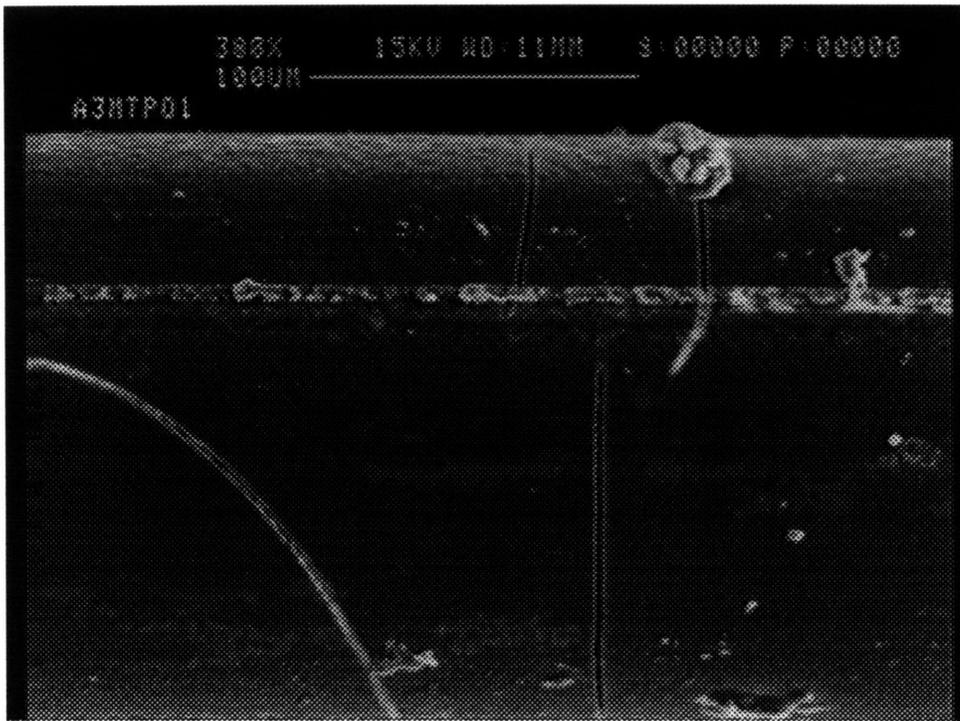
Figure 6-110: The Acrylate-coated optical-fiber 3 month inside the cement paste (pull-out extraction).
