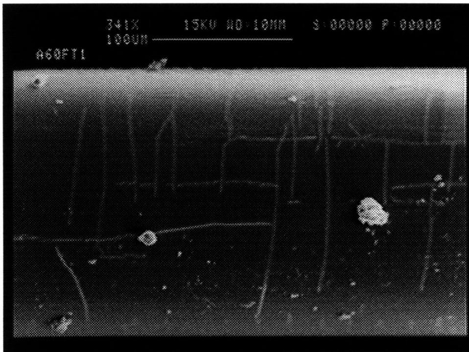
Figure 6-106: The Acrylate-coated optical-fiber under 60 freeze-thaw cycles (341 X).
